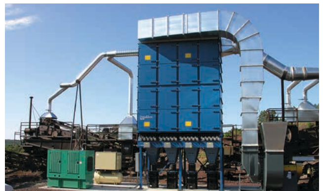
DLMC on Rock Crushing 41,000 cfm (69,645 m 3 /h)
