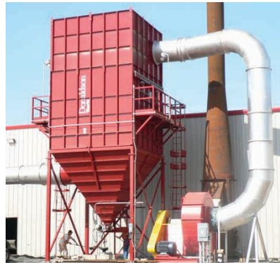
MB on Glass Processing 25,000 cfm (42,466 m 3 /h)
