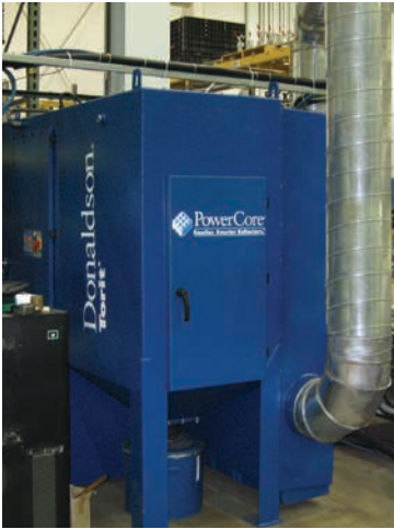
TG on Plasma Cutting 2,300 cfm (3,90 m 3 /h)
