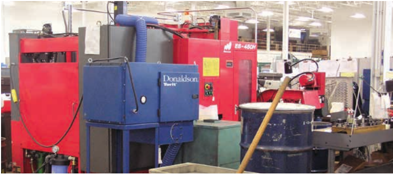
DMC on Machining 800 cfm (1,359 m 3 /h)
